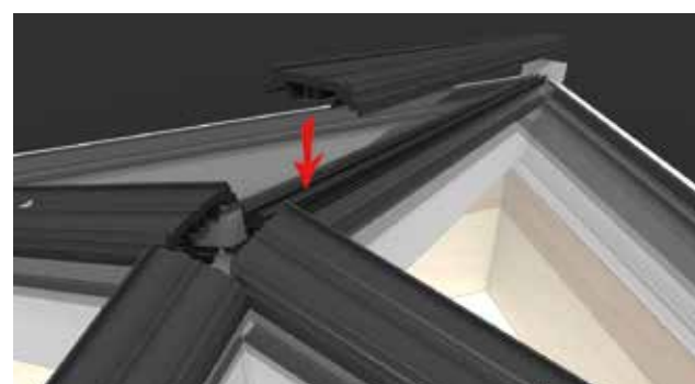
18 Fit the shorter pressure plates after the longer pressure plates have been secured.
