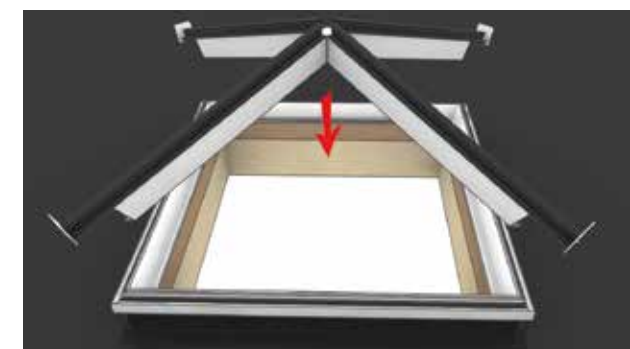
11 Once all the rafters are secured to the box ridge drop the assembled frame onto the ringbeam pushing the hips tight into the corners.
