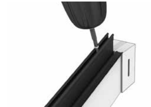
9 Re-tighten the screw on the top of the hip rafter making sure the joint is tight.
