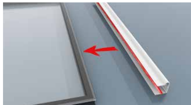
15 Apply a bead of sealant to glazing end closer and fit centrally to glass units. Note: Always use the correct polymer sealant for self cleaning glass. Illustration shows underside of glass, note when fitting, drip faces down.
